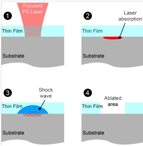
**Figure 2** Laser spallation schematic where (a) a focused laser beam is absorbed at an interface (b) heating occurs in a thin layer (c) a shock wave expands (d) the thin film layer is removed.
