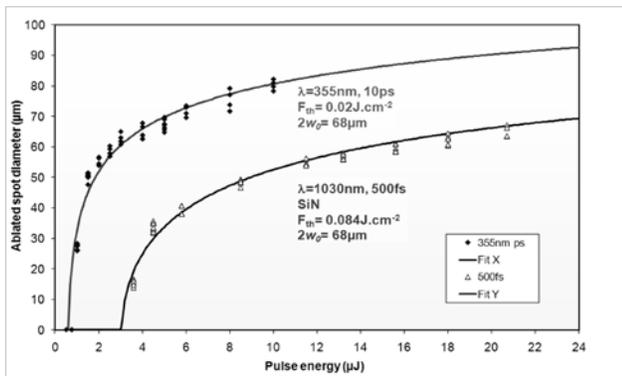
**Figure 6** Comparison of 355 nm picoseconds and 1030 nm femtosecond laser ablation thresholds for removal of thin film SiN.
