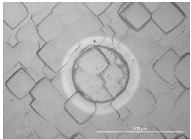
**Figure 8** Single pulse 532 nm removal of Al<sub>2</sub>O<sub>3</sub>/SiN backside passivation layer to produce 65 μm diameter contact hole.
