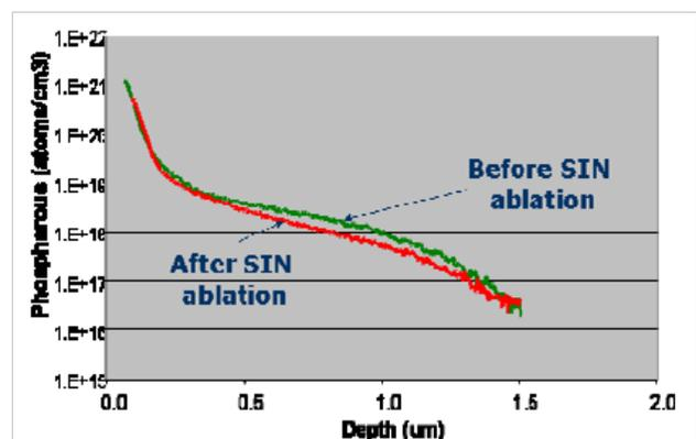
Figure 5 Emitter dopant profile before and after laser ablation of SiN using 355 nm picosecond pulses on a textured Si wafer [9].
