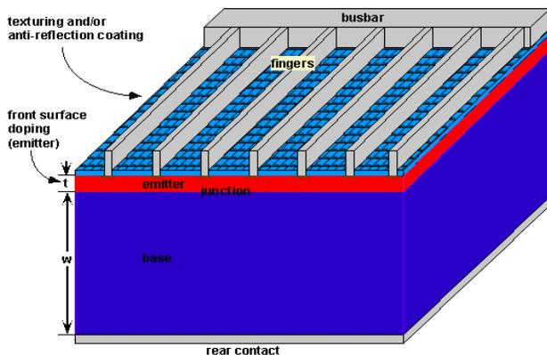
**Figure 1** Simplified schematic of a silicon solar cell with front-side finger and busbar pattern.
