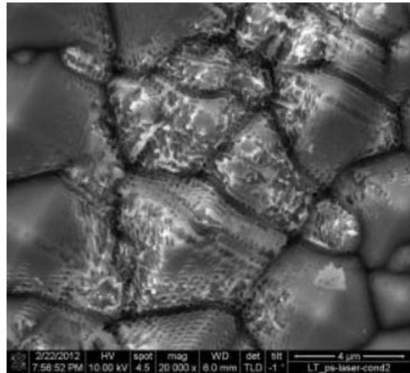
Figure 4 SiN scribing using ( $\sim 1.4 \cdot F_{Th}$ ), 355 nm pulses at a scan speed of 4 m/s [8].
