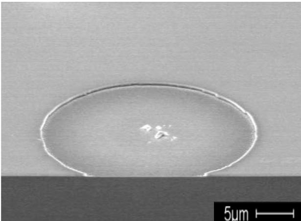
**Figure 7** Removal of a SiO<sub>2</sub> from silicon using 355 nm picosecond pulses at an optimum fluence of  $\sim 0.11 \text{ J/cm}^2$  ( $\sim 1.5 \cdot F_{Th}$ ).
