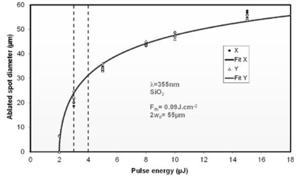
**Figure 3** Laser ablation threshold curve for a 100 nm thick  $\text{SiO}_2$  thin film on silicon using 355 nm picosecond pulses. The dashed lines indicate the optimum removal regime.
