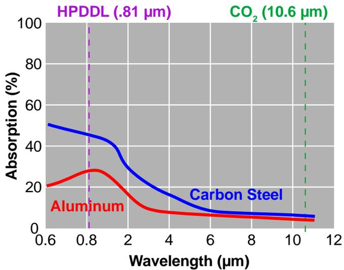
*Absorption as a function of wavelength for carbon steel and aluminum*
