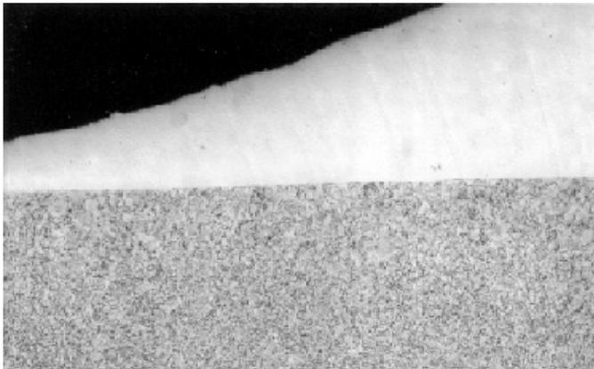
SEM photo of the clad cross section shows essentially no dilution of the substrate material
