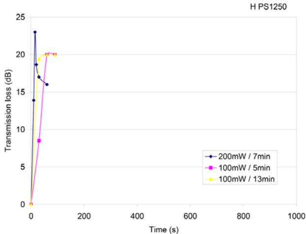
**Figure 6.** Grating growth in hydrogen-loaded PS1250
