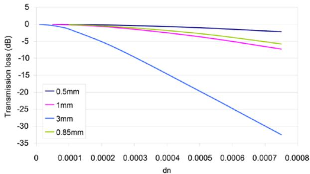
**Figure 9.** Variation of transmission loss vs.  $dn$  for various grating lengths
