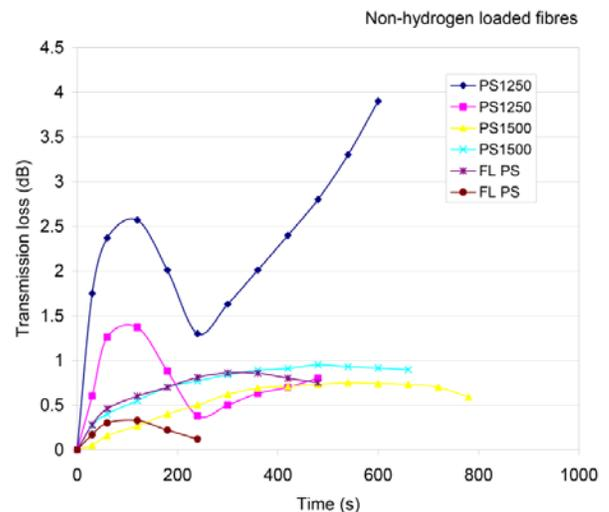
**Figure 8.** Grating growth in non-hydrogen-loaded fibers
