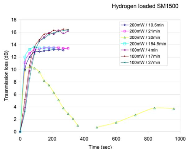
Figure 5. Grating growth in hydrogen-loaded SM1500
