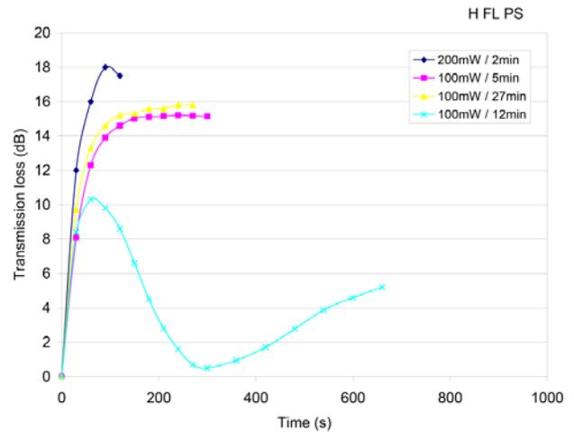
**Figure 7.** Grating growth in hydrogen-loaded Fiberlogix PS
