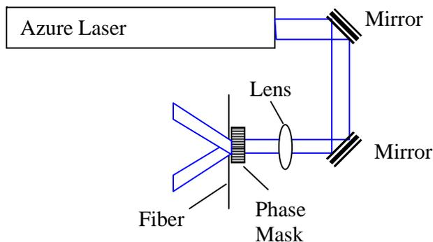
Figure 3: Schematic of the grating fabrication arrangement.
