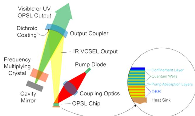
**Figure 1. Schematic illustration showing the main components of an optically pumped semiconductor laser (OPSL), such as a Coherent Sapphire.**
