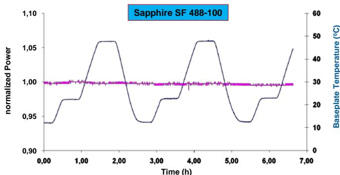
**Figure 4.** The output power of Sapphire SF lasers is very stable and completely unaffected by even large changes in ambient temperature.
