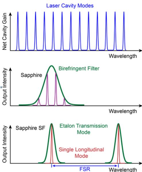
**Figure 3.** An additional frequency-selective element is incorporated within the Sapphire SF cavity in order to constrain laser operation to a single longitudinal mode, resulting in an output linewidth <1.5 MHz.
