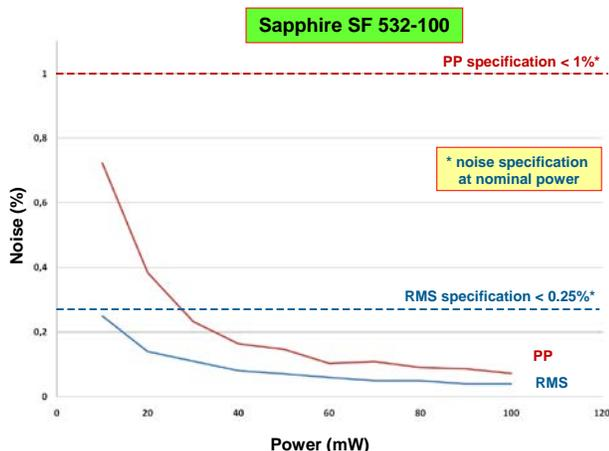
**Figure 5.** The output noise of Sapphire SF lasers is far below the 0.25% specification at maximum output power and at nearly every other power level.
